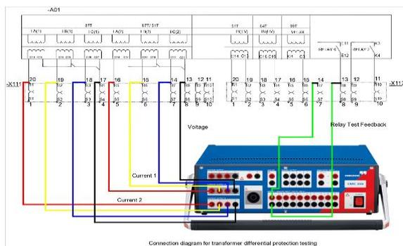
Fig. 2: SEQ Fig. \\* ARABIC 2 Differential wiring connection
