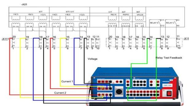
Fig. 3: Over fluxing protection scheme
