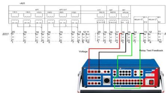
Fig. 4: SEQ Fig. \\* ARABIC 4 Overcurrent protection scheme
