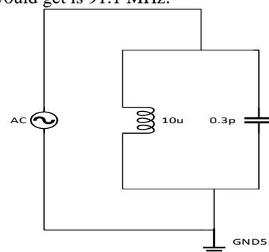
Fig 5 tank circuit design
