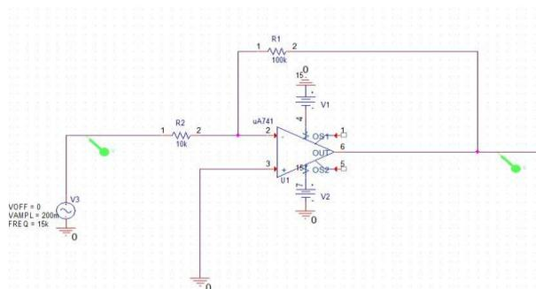
**Fig 6** Audio amplifier simulation circuit
