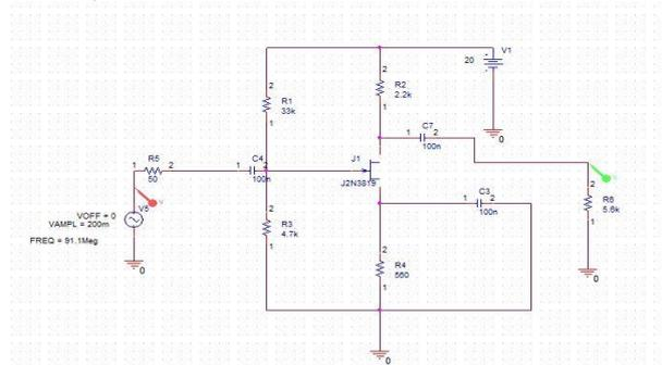
Fig 3 Simulation circuit of RF amplifier
