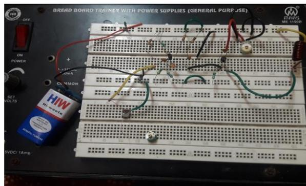
**Fig 8** Breadboard implementation of FM Transmitter circuit.
