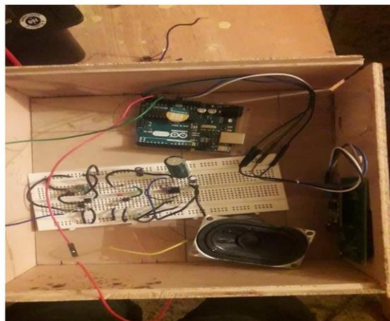
Fig 12 Fabricated FM Receiver.
