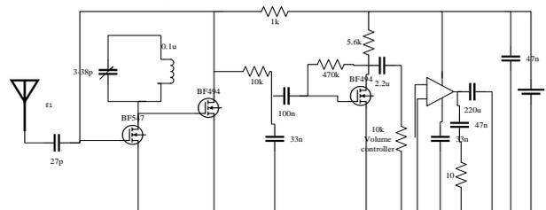
**Fig 2** FM Receiver circuit.
