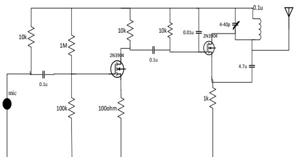
**Fig 1** FM Transmitter circuit.
