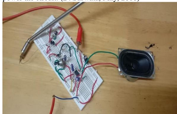
**Fig 9** Breadboard implementation of FM Receiver circuit.
