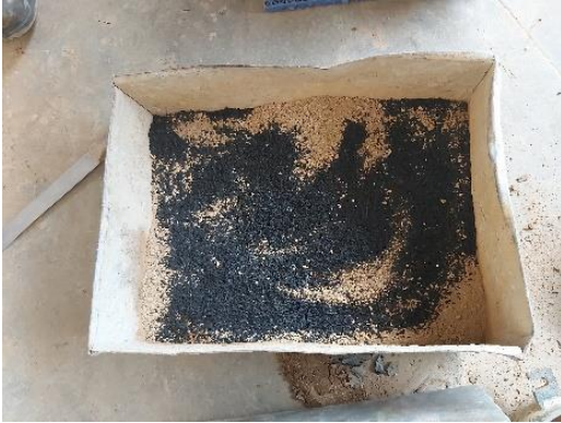
Fig.6 Soil-tyre crumb mix
